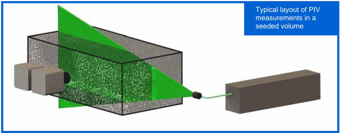
Typical layout of PIV measurements in a seeded volume
